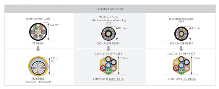
\*Corning's patented Binderless\* FastAccess® technology refers to the combination of a Corning FastAccess technology jacket with an innovative technology used to bind cable construction through the manufacturing process, eliminating the use of binder yarns and waterblocking tapes.
